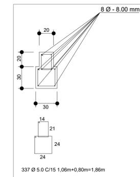
DETALHE SAPATA CORRIDA SEM ESCALA
