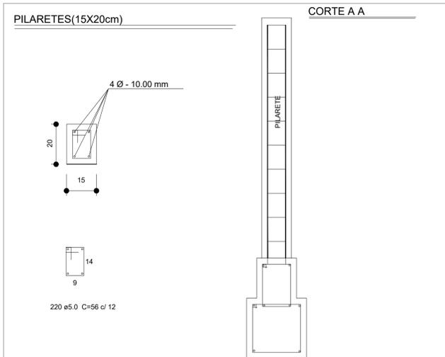
DETALHE PILARETE MURO SEM ESCALA
